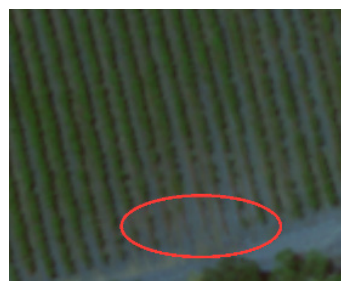
Fig. 2. Missing vines at the row-end of a vineyard block results in misrepresentation of end-post location
