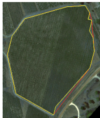
Fig. 1. Convex Hull (red) of a vineyard block which does not follow actual block outline (yellow)
