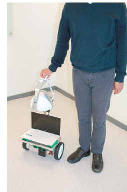
Fig. 1. Human-friendly walking assisting robot vehicle ( hWALK ) developed at Karlstad University.
