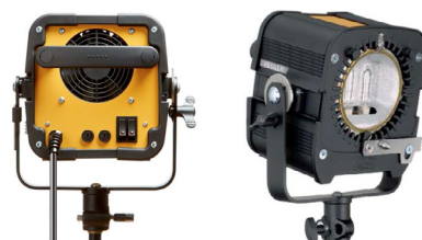
Figure 3: The Hedler IR excitation source used in the IR experiments
