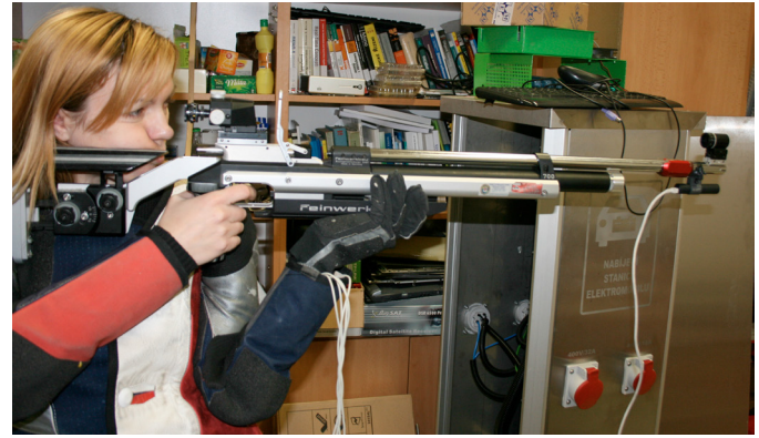
Fig. 3. Preparing for measurement: SCATT optical sensor is mounted on the end of the barrel
