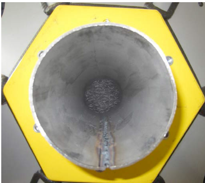
Fig. 2. Electromagnetic mill working chamber (visible grinding media).
