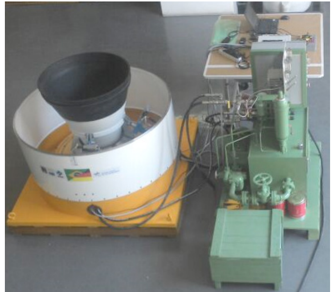
Fig. 4. Mockup of rocket motor nozzle with aft skirt including the actuation system
