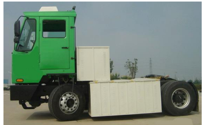
Fig. 1. The supercapacitor truck.
