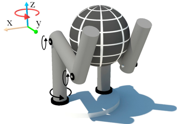
Fig. 1. A 6-DOF cooperative whole arm manipulator enclosing an object.
