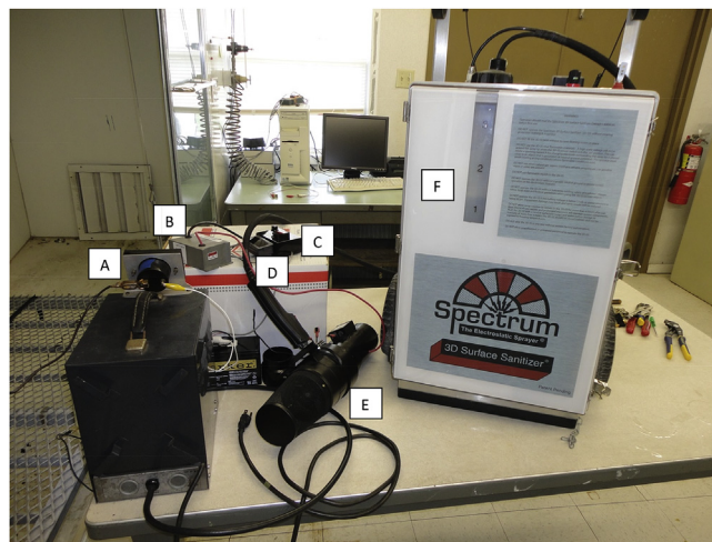
Fig. 2. The Electrostatic sprayer (3D Surface Sanitizer) used in the study for spraying ryegrass. Shown in the photo are A) Microammeter, B) +10 kV power supply, C) Voltage regulator, D) LED voltage display, E) Spray gun with integrated nozzle, and F) Electrostatic spray unit with spray tank, Power switch, Pressure gauge, Pressure regulator, Battery and diaphragm pump.
