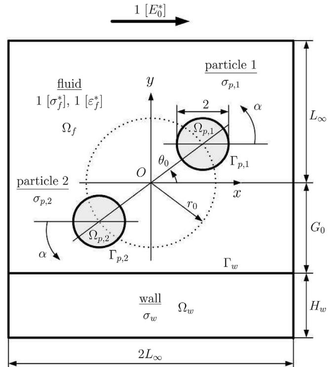
Fig. 1. Non-dimensional schematic diagram of the flow geometry and computational domain.
