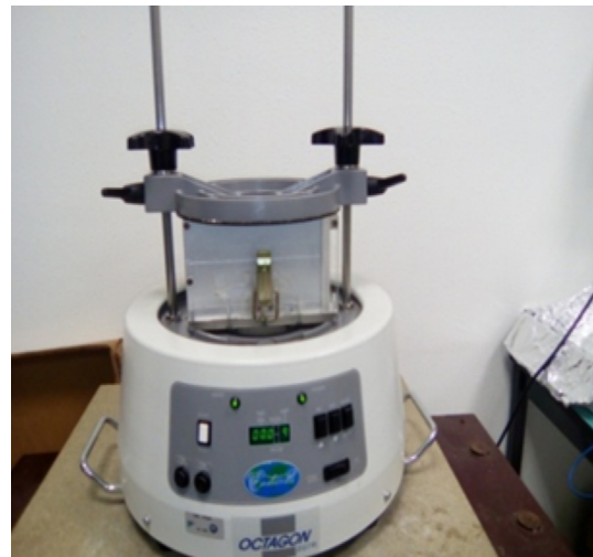
Fig. 2. Photography of the vibrating system for triboelectric charging of granular material.
