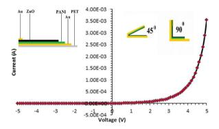
**Fig. 3.** Dark I - V characteristics of ZnO/PANI heterojunction measured at 300 K, in flat and bending condition at an angle of 45° and 90°. Inset shows the schematic of the diode.
