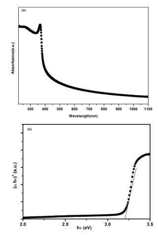
Fig. 2. (a) UV-visible absorption spectra of ZnO film (b) determination of band-gap energy.
