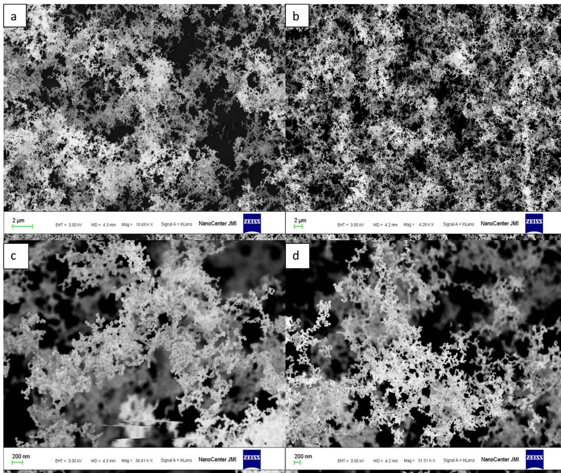
Fig. 1. (a-d): FESEM Images of as-deposited  $\text{Pb}_5\text{Se}_{95-x}\text{Zn}_x$  film with  $x=10$ .
