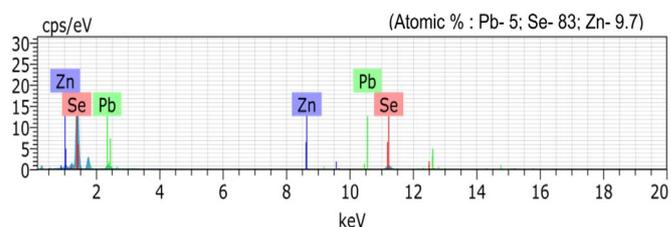
Fig. 2. : EDAX Image of as-deposited  $\text{Pb}_5\text{Se}_{95-x}\text{Zn}_x$  thin film with  $x=10$ .
