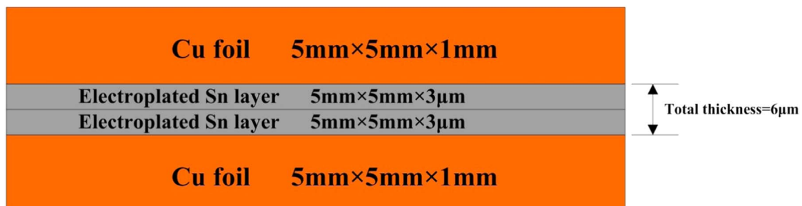
Fig. 1. Schematic illustration of Cu-6 \mu\text{m} Sn-Cu sandwich structure..
