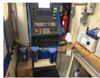
c) Silica gel boxes and data acquisition systems (APS, SMPS)
