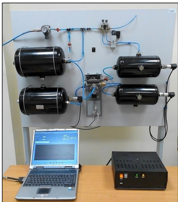
Fig. 1. The test apparatus for determination of static characteristics of brake valves.
