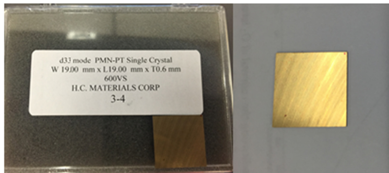
Fig. 1. PMN-PT single crystal plate resonator.
