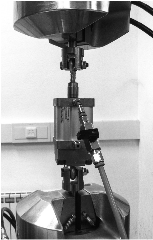
Fig. 1. Pneumatic linear actuator characterised for the case study.
