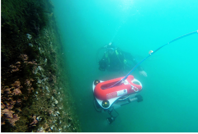
Fig. 1. View of the L2ROV underwater vehicle. Its six thrusters allow precise control of its 6 degrees of freedom.
