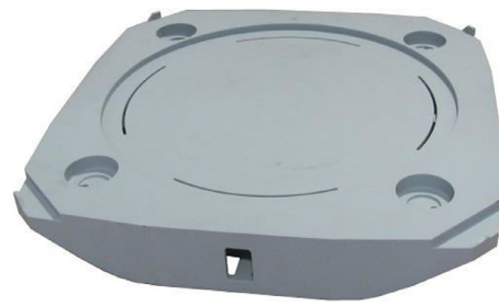
Fig. 1. A photograph of an experimental stage design made of ceramics.
