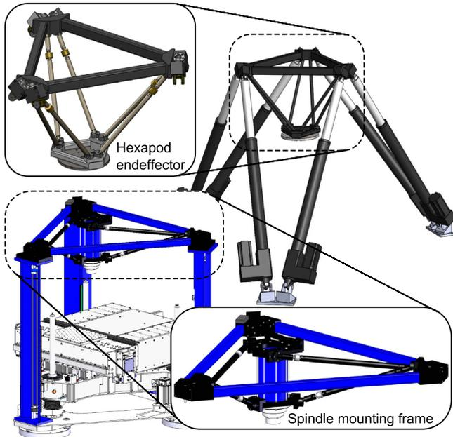
Fig. 2. Light-weight rigid bar frameworks in machines, particularly suitable for force sensor integration; above: end-effector of hexapod FELIX (moving), below: spindle mounting frame of experimental machine MAX (not moving)
