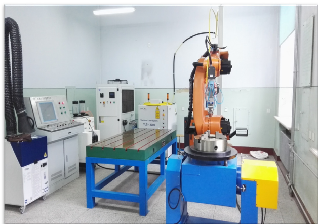
Fig. 1. Laser cladding system for laser cladding/remelting processing.
