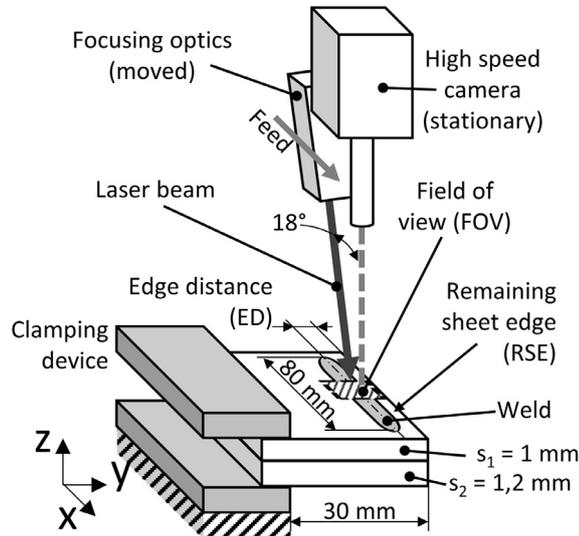
Fig. 2. Experimental setup.
