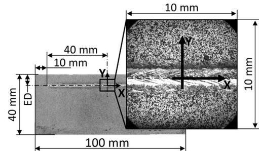
Fig. 4. Field of view (magnified) and its location on the sample.
