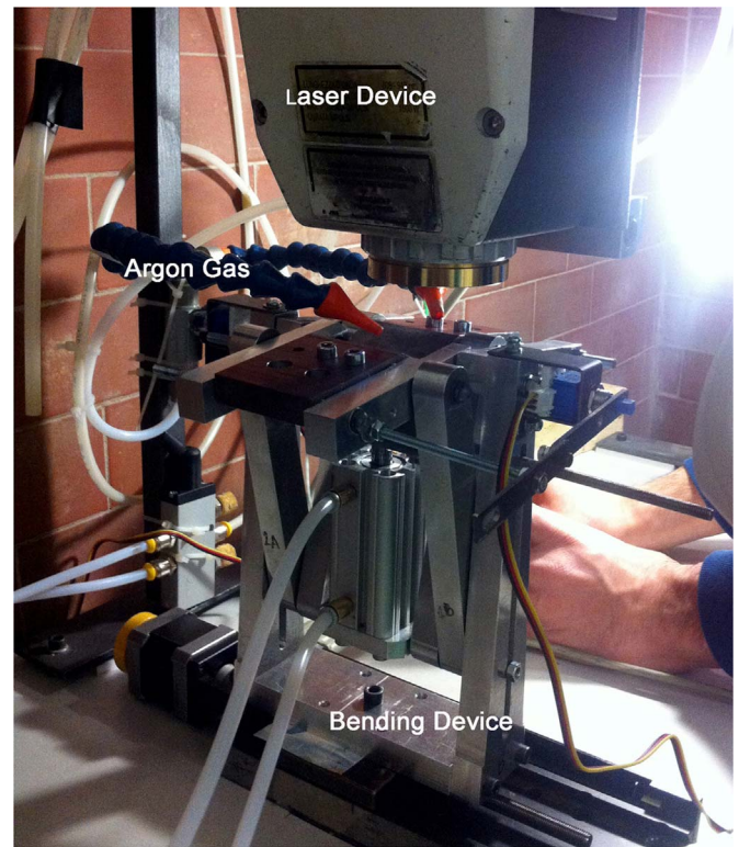
Fig. 1. Laser head and auxiliary bending device with the clamping device to hold the workpiece during external force laser-assisted bending process.
