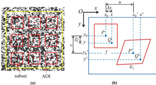
Fig. 1. Displacement field representation using rectangular subsets. (a) partitioning of the area of interest (AOI). (b) displacement representation of one subset.
