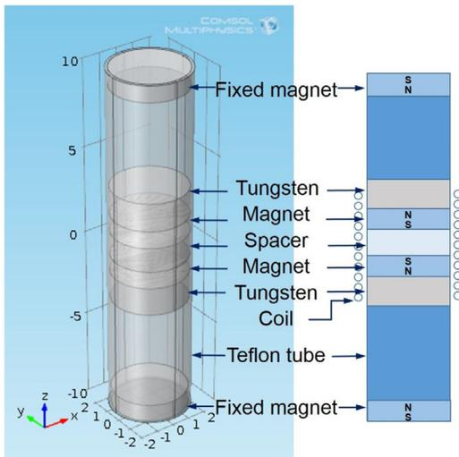
Fig. 1. Schematic of magnet levitated harvester [11].
