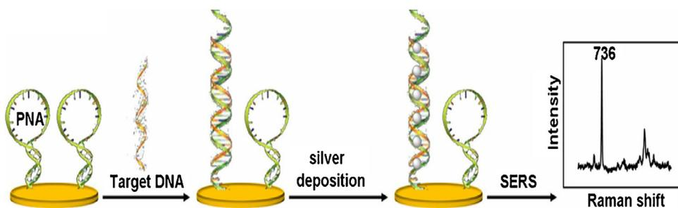
**Scheme 1.** Schematic illustration of label-free and Raman dyes-free SERS strategy used for DNA detection.
