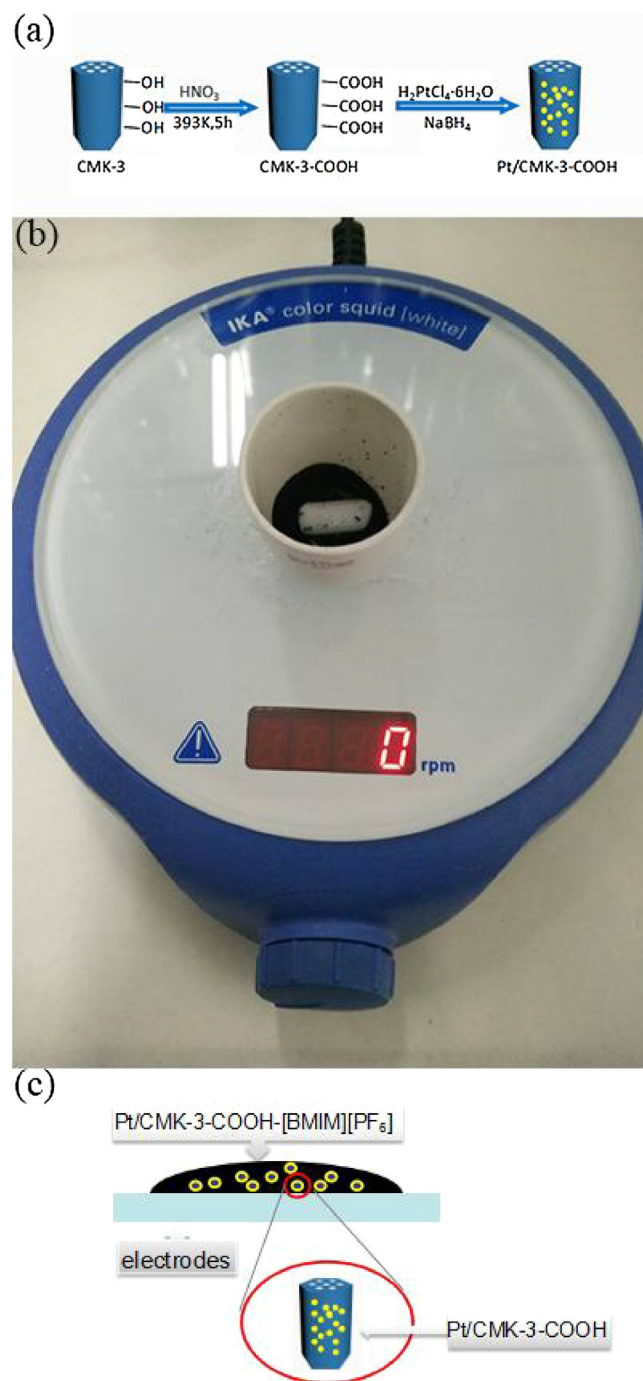
Fig. 1. Scheme of preparation for Pt/CMK-3-COOH (a); Procedure of mixing Pt/CMK-3-COOH with [BMIM][PF 6 ] (b); Illustration of the structure of O 2 sensor (c).
