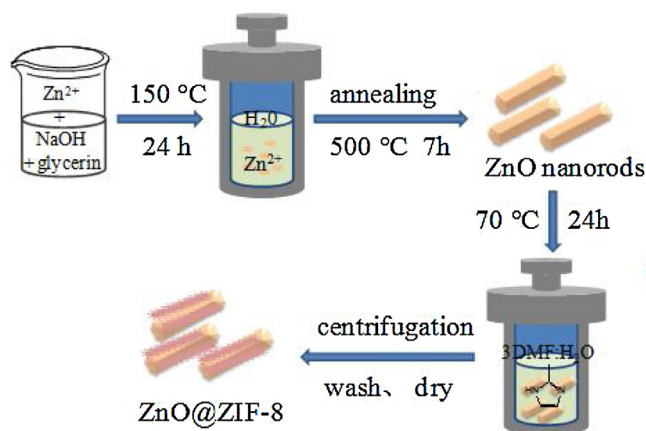
Scheme 1. The illustration of the procedure to synthesize ZnO@ZIF-8.
