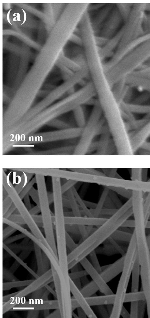
Fig. 1. SEM images of (a) pristine and (b)  $\text{In}_2\text{O}_3$  nanoparticle-decorated ZnS nanowires.
