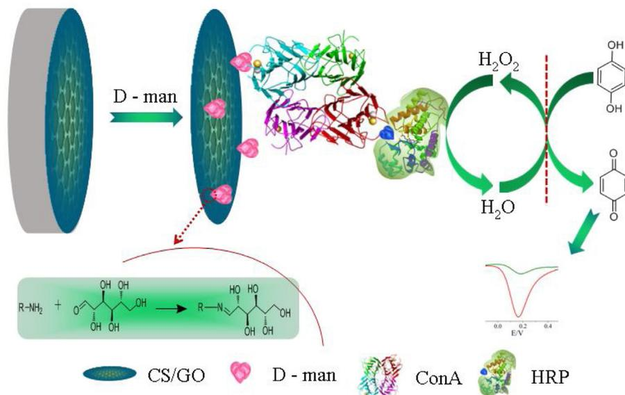
**Scheme 1.** Construction of a novel sandwich electrochemical sensor for determination of ConA.
