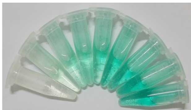
Fig. 1. a: Photographs for various concentrations of \text{H}_2\text{O}_2 (from left to right: 0, 3.4 \times 10^{-7} , 1.7 \times 10^{-6} , 3.4 \times 10^{-6} , 1.7 \times 10^{-5} , 3.4 \times 10^{-5} , 9.5 \times 10^{-4} , 3.2 \times 10^{-4} , 9.7 \times 10^{-3} , M) and TMB reaction solution catalyzed by EDTA. b: Typical absorption spectra of the produced TMB corresponding to (a).
