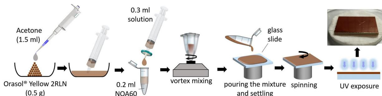
Fig. 1. Illustration of the process steps in fabrication of the filters.
