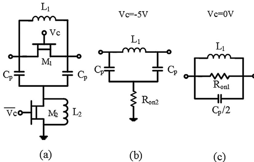
Fig. 1. (a) Topology of the switched filter. (b) Equivalent circuit when  $V_c = -5\text{V}$ . (c) Equivalent circuit when  $V_c = 0\text{V}$ .
