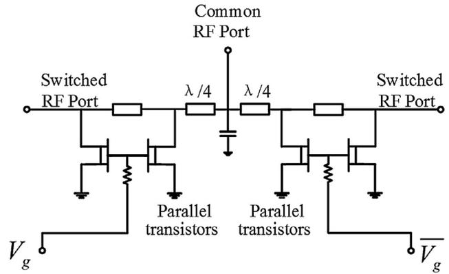
Fig. 2. The shunt configuration of AlGaIn/GaN SPDT.
