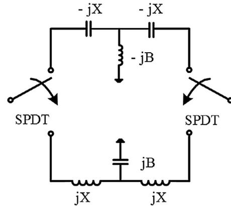
Fig. 3. The schematic of the T-type high-pass/low-pass.
