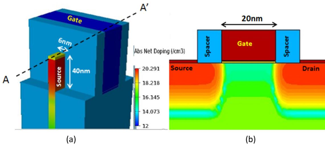
Fig. 2. (a) Structure of the 3D nFinFET modeled in this work; (b) cross section along AA’ showing source-drain and channel doping concentrations labeled in logarithmic scale.
