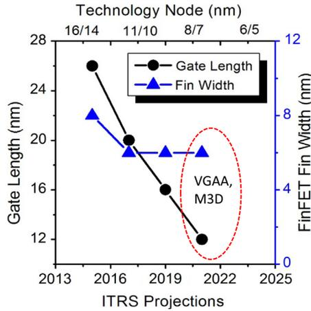
Fig. 1. Projected fin width and gate length for upcoming technology nodes [9].
