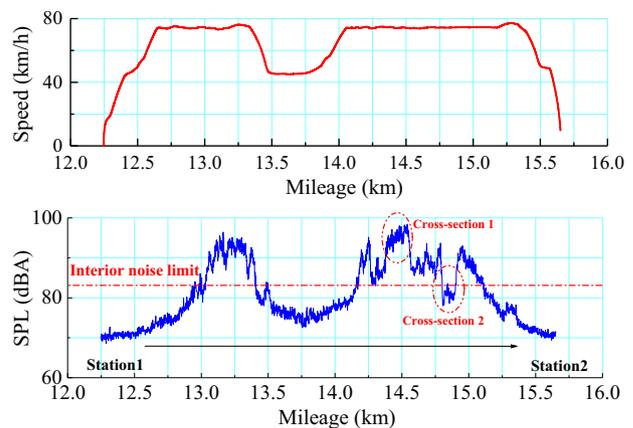
Fig. 2. Interior noise and speed vs. mileage.
