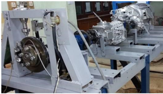
Fig. 1. Photo of brake dynamometer test setup and measurement instrumentation.
