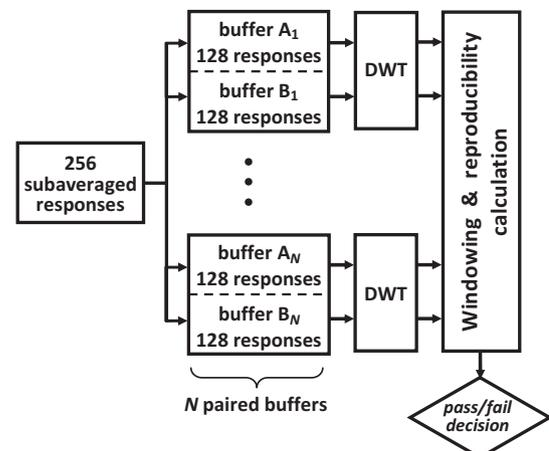
Fig. 1. Block diagram of the proposed wavelet-based algorithm.
