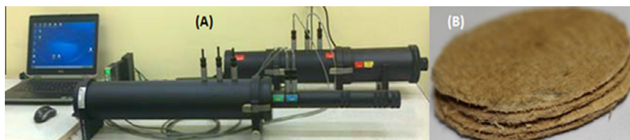
Fig. 1. Sound absorption measurement procedure: (A) Brüel&Kjær impedance tube set up; (B) sample of the barkcloth layers studied.
