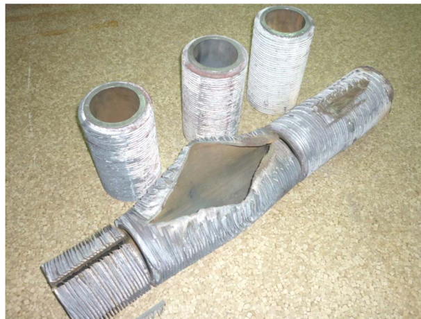
Fig. 2. Appearance of the failed sample evaluated in the lab.
