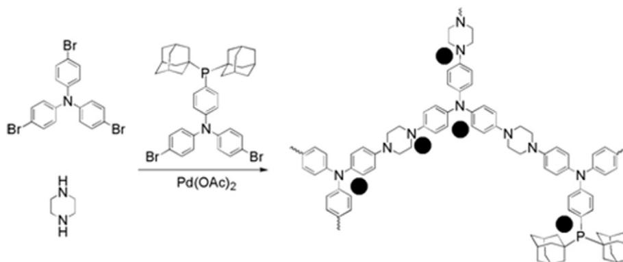
**Scheme 1.** The preparation of the Pd@NPd<sub>2</sub> catalyst.
