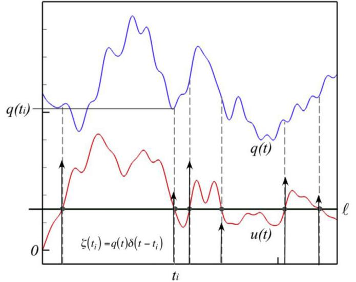
Fig. 1. Level crossings of the signal  $u$  marked by the random quantity  $q$ .
