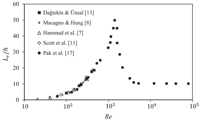
**Fig. 1.** Published results of shear layer reattachment length versus flow Reynolds number for  $Er = 2.00$ .
