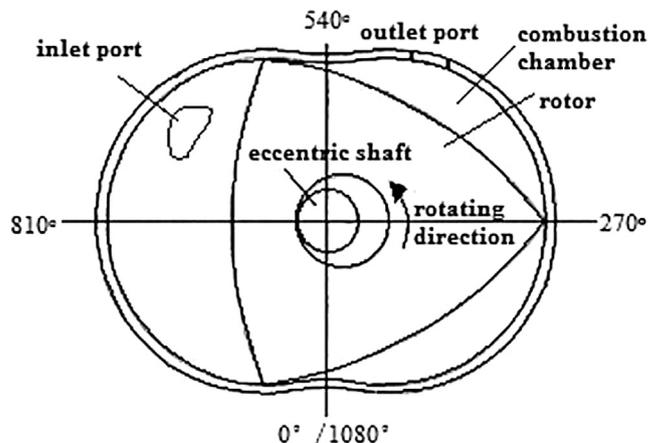
Fig. 1. Schematic of the tested rotary engine.
