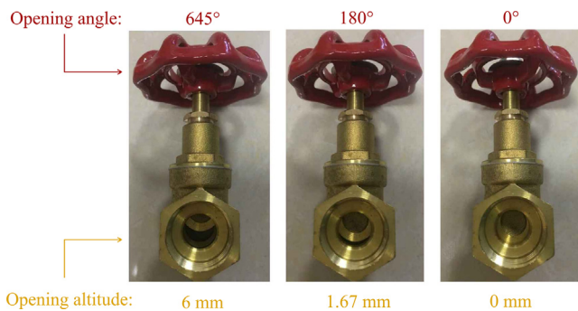
Fig. 1. Gate valve at different open positions.
