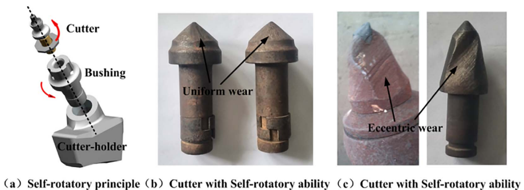
Fig. 2. Self-rotatory principle and wear condition of cutters with different self-rotatory ability.
