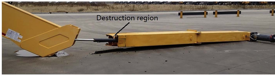
Fig. 1. Instability example of retractable outrigger.
