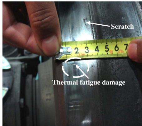
Fig. 1. Typical thermal damage on the high-speed wheel tread [12].
