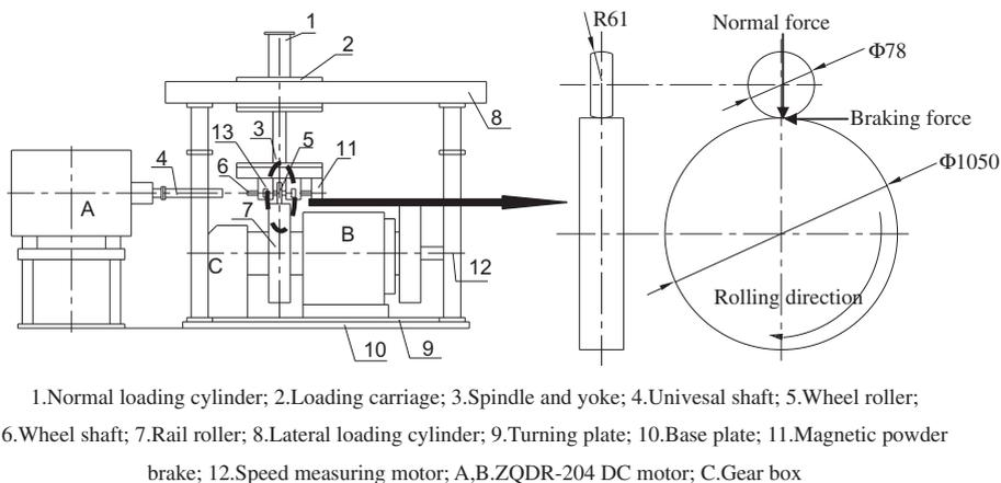
Fig. 2. Wheel/rail simulation apparatus and simulating wheel and rail rollers. 1. Normal loading cylinder; 2. Loading carriage; 3. Spindle and yoke; 4. Universal shaft; 5. Wheel roller; 6. Wheel shaft; 7. Rail roller; 8. Lateral loading cylinder; 9. Turning plate; 10. Base plate; 11. Magnetic powder brake; 12. Speed measuring motor; A, B. ZQDR-204 DC motor; C. Gear box.
