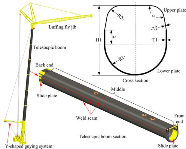
Fig. 1. A TBS of the all-terrain crane.
