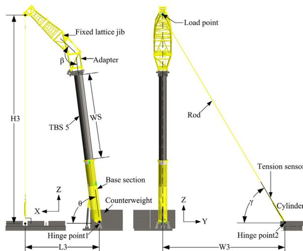
Fig. 2. Sketch of experimental structure.
