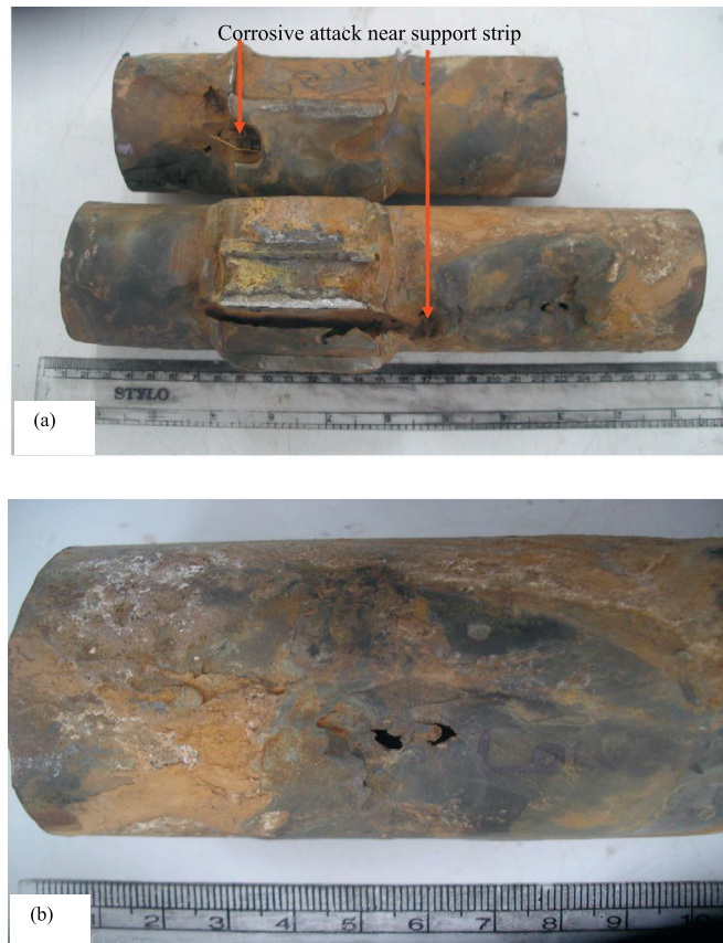
Fig. 1. (a) Failed cooling coil tubes in as received condition. (b) Close visual observation near the failure.
